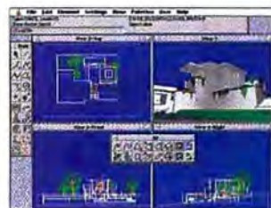
THE FOUR-WINDOW VIEW OF AN UNUSUAL BUILDING BEING DESIGNED IN VERSION 4.2 OF MICROSTATION.
