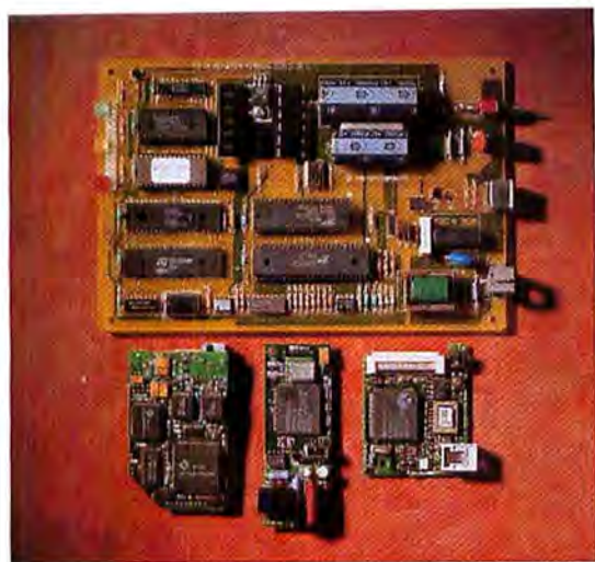
Ever-smaller computers require ever-smaller modems. Compare the modem board from the external Shiva Netmodem/E (top) to those used in the Outbound Pocket Port Fax Modem external fax modem (lower left), Apple PowerBook 170 internal modem (center), and PowerBook Duo internal modem (right).
