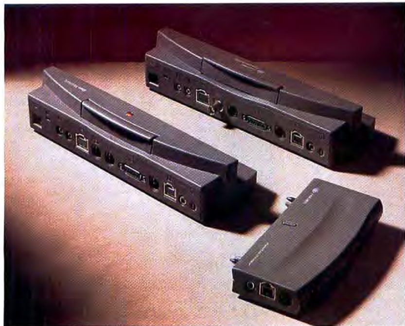
The PowerBook Duos introduced revolutionary docking stations, including E-Machines' PowerLink DeskNet (top), which adds Ethernet connections; E-Machines' PowerLink Presenter (right), which adds extensive video connections; and Apple's MiniDock (left), which offers standard Mac connections.
