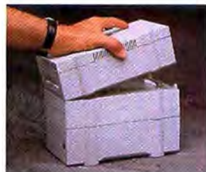
THE SMARTSTACK FROM ENVIVIO CAN STACK AS MANY AS SEVEN SCSI MODULES.
