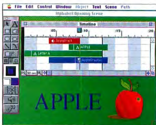
Action's Timeline Window Bars on the time line give you second-by-second control over each object and event in a scene. Here, two text objects (one hidden behind the Timeline window), a PICT graphic, and a sound file, have been combined to create a 12-second scene.
