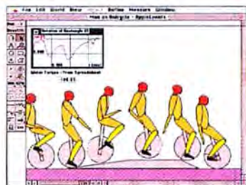
UNICYCLE PHYSICS. WORKING MODEL CAN EXPORT DATA IN REAL TIME FROM THE MODEL TO GRAPHING OR OTHER PROGRAMS.
