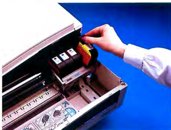
The Canon CJ10 is designed to be virtually maintenance free, with Bubble-Jet cartridges that contain all the important components.
