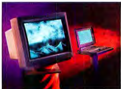
THE 19-INCH MONOCHROME TWO-PAGE SCSI DISPLAY FROM LAPIS CONNECTS DIRECTLY TO A SCSI PORT.
