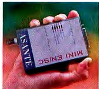
ASANTÉ'S MINI EN/SC IS A PORTABLE SCSI-TO-ETHERNET ADAPTER THAT WEIGHS ONLY 6 OUNCES.
