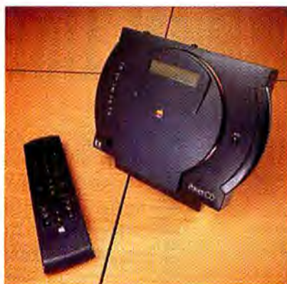
APPLE'S POWERCD PLAYS CD-ROM, AUDIO, AND PHOTO CD DISCS ALL FROM ONE SMALL PACKAGE.
