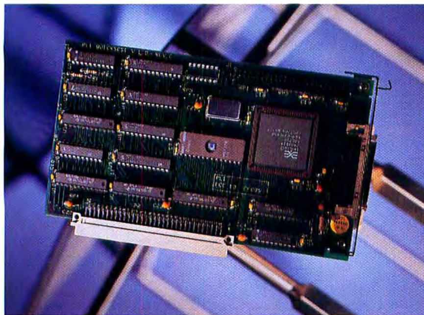
The PLI QuickSCSI SCSI adapter, which lists for only $499, was the fastest we tested.
