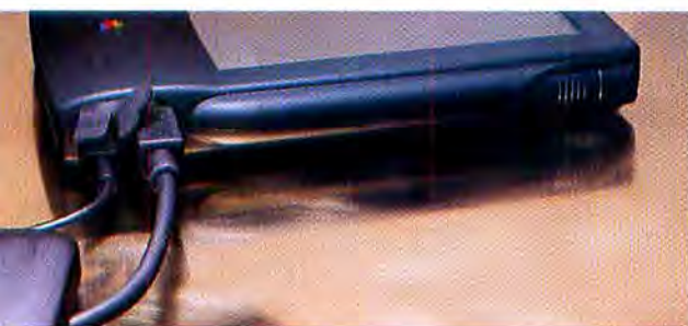
Newton's Versatile Ports Newton offers storage expansion with a PCMCIA slot (with card inserted, top photo), and connectivity through an infrared remote-control transceiver (to the left of PCMCIA slot) and a serial port (bottom photo, far left, with cable inserted). An AC adapter port (bottom photo, with power cord inserted) sits between the serial port and the pen carrier.
