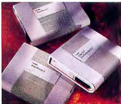
Farallon's routers, the StarRouter (top left) and the InterRoute/5 (bottom left), and hub, the Ether10-T StarController/557 (right), support SNMP and AURP protocols.
