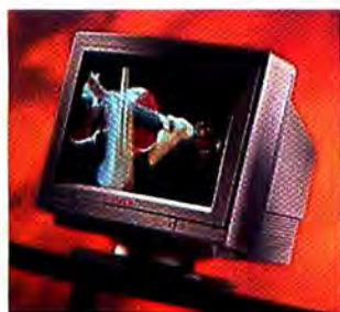
Mirror's ProView 14-inch Multimedia Color Display has stereo speakers on its sides.
