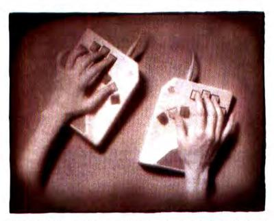
The Bat uses a process called chording-entering each character based on a combination of keystrokes-to achieve significant ergonomic improvements, according to Infogrip, which sells the unusual-looking device.
