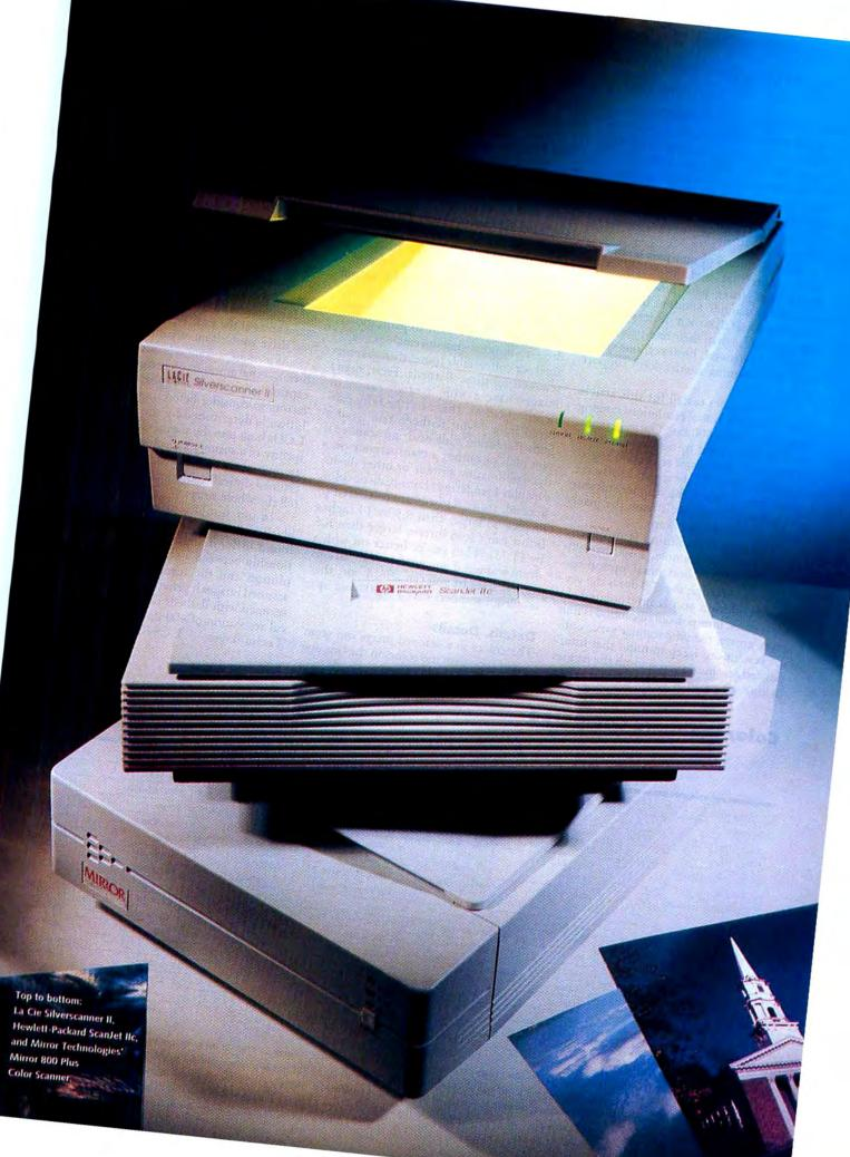
head (which contains the CCDs) passes over an image only once to capture the RGB data. Three-pass scanners typically employ one lamp and three color filters; the scanner head moves across an image three times, once while the red filter is over the lamp, again while the green filter is in place, and again while the blue is in place.
