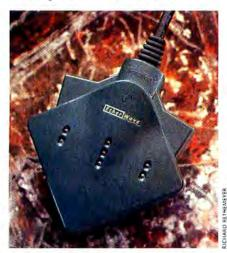
Farallon's Etherwave three-port repeater connects nodes easily with modular phone cable.
