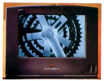
The PowerBook Duo 250 features a monochrome active matrix display (above left). The 270c (above right) uses a color active matrix screen; here, it is display-
