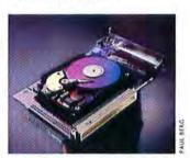
The ETC Peripherals Purple Bullet board accepts a 31/2-inch hard drive and fits in a NuBus slot.
