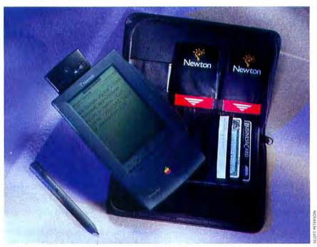
Communications applications for the Newton MessagePad make it more than a finicky steno pad. Here, the Messaging Card turns the Newton into a pager that can receive messages of up to 240 characters—verbose compared with the usual pager messages. The card can store 120K worth of messages at a time.
