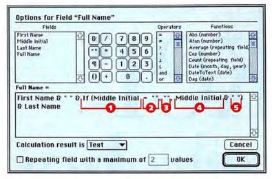
Calculating Text FileMaker's Field Options dialog box shows a calculation that combines the first-name, middle-initial, and lastname fields into the new full-name field. The If function (1) tests the middle-initial field to see if it is empty (2); if so, the function enters nothing (3) in the fullname field. If it finds a value (4), it enters that value and follows it with a blank space (5).
