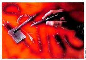
The Wedge-One bar-code reader with its ADB interface (left), and the wand-only Scan-One. Both use HP wands.
