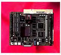
The logic board of the LC 575 includes a new communications slot (on upper right).
