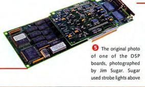
and below the board together with a gold reflector (which bounced light onto the board to give it a golden cast); he scanned the photo at high resolution with a Leaf scanner.
