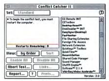
Automated INIT Testing Casady & Greene's Conflict Catcher II can automatically test groups of INITs to pinpoint which ones are causing problems.
