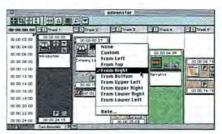
On the Right Path In the Pro version of Passport Producer, you can make objects fly into view along a path. A pop-up menu on each cue tile allows you to set the direction of the path and the rate at which the object will move.
