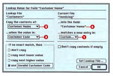
Look It Up The logic of FileMaker's Set Lookup dialog box runs clockwise from the bottom right. Data entered in the Invoicing file's customer-code field (1) is compared with the Customers file's customer-code field (2). If they match, the Customers file's Customername field (3) is copied back into the Invoicing file's customer-name field (4).
