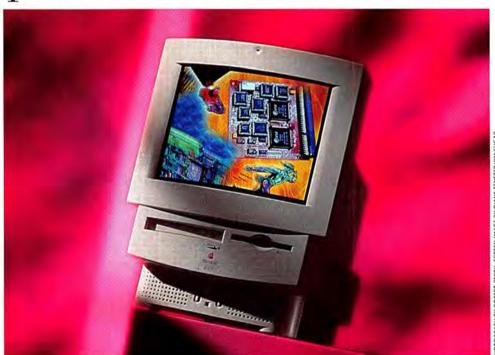
With a 33MHz 68LC040 microprocessor, Apple's Macintosh LC 575 is the fastest all-in-one Mac ever (see the benchmarks, "How Fast Are the LC 550 and 575?" on page 38).
