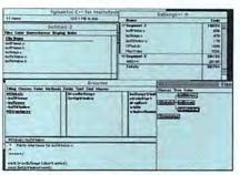
**Looking Up** The editor in Object Master's Browser window supports a Find And Paste Method Call command that looks up parameters for you in OM's data dictionary. This not only saves time but helps avoid trivial errors.
