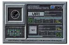
Confidence Testing Programs Programs like MicroMat's MacEKG can check a Mac's hardware components to see if their performance matches Apple's specifications. That sometimes helps narrow down possible causes of problems.
