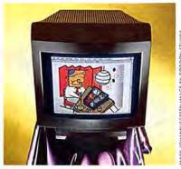
The Apple Multiple Scan 20 Display uses a 0.31mm stripe-pitch Trinitron tube and can show resolutions from 640 by 870 pixels up to 1280 by 1024 pixels.
