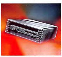
PLI's Infinity 270 Turbo uses SyQuest's latest, a 3.5-inch, 270MB removable-cartridge drive called the SQ3270S.
