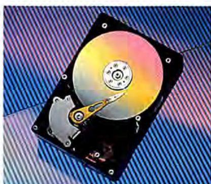
Quantum's Grand Prix 4280 hard drive stores 4GB of data and has an average access time under 9ms.
