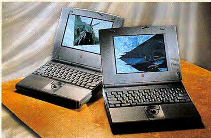
Faster Duos The new PowerBook Duo 280 and 280c look the same as the Duo 250 and 270c, which they replace. However, a 68040 CPU makes the new Duos considerably faster than previous models.
