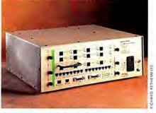
Cabletron's communications hub has room for up to 28 modems.
