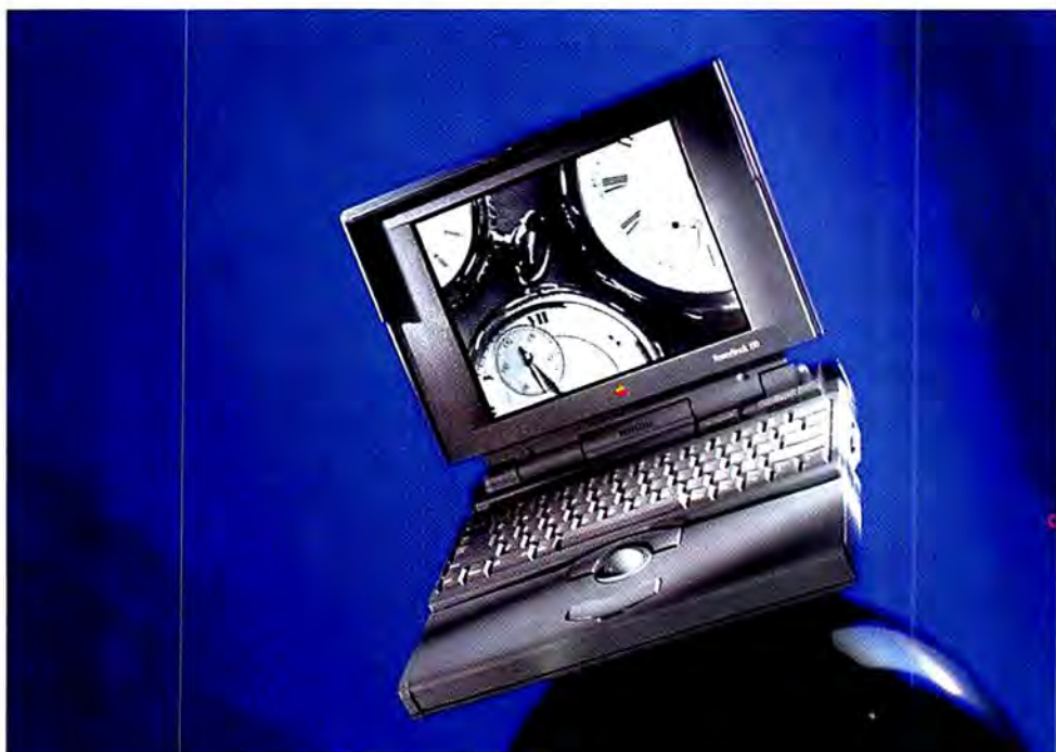
Apple's latest portable, the PowerBook 150, weighs about a pound less than previous all-in-one models but still uses a 68030 processor (see the benchmarks, "PowerBook 150: How Fast Is It?," on page 34).
