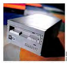
FWB's HammerDisk PE230 is an erasable optical drive with removable 230MB cartridges.
