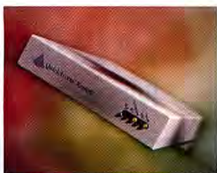
AccessWorks' QuickAccess Remote, an ISDN digital modem that costs less than $500, has one 115.2-Kbps data port.
