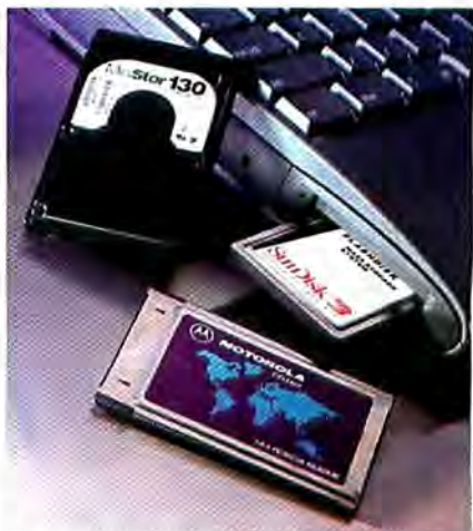
The installed PCMCIA module with More's Mini-Stor 130MB drive, Sundisk's 1.8MB flash disk, and Motorola's CELlect 14.4 fax modem.
