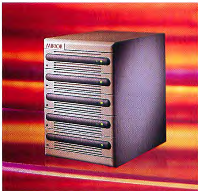
Mirror's RAID systems, such as the Precision 6, feature unique slide-out trays that include both a drive mechanism and a power supply.
