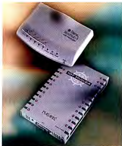
The DaynaStar MiniHub-5 (top) takes up little more space than a stack of index cards, and Asanté's 10T Hub/24 about twice that amount.
