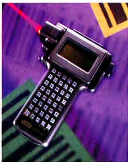
The OmniWand bar-code reader also has a keypad for entering data not captured in the bar code.
