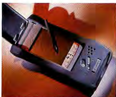
The SuperTech 2000 is a ruggedized PDA that uses Apple's Newton technology.
