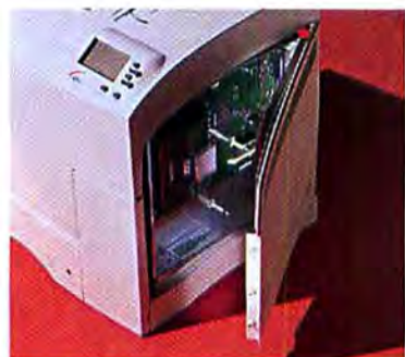
A hinged door on the side of the Lexmark Optra series printers eliminates screws, making it easy to add memory or other upgrades.
