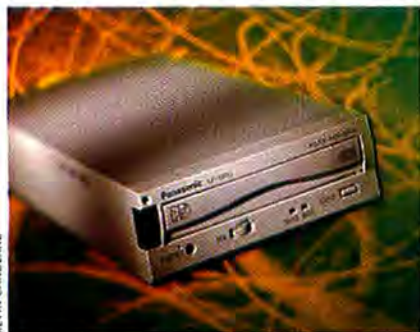
Panasonic's new quad-speed CD-ROM drive can also read and write a new type of 650MB optical disk.
