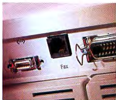
A telephone jack for a PostScript fax modem on the Apple LaserWriter 16/600 PS enables the printer to receive and print faxes.
