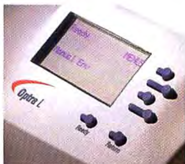
Front-panel buttons and an LCD display provide easy-to-use menus for controlling the Lexmark Optra series.
