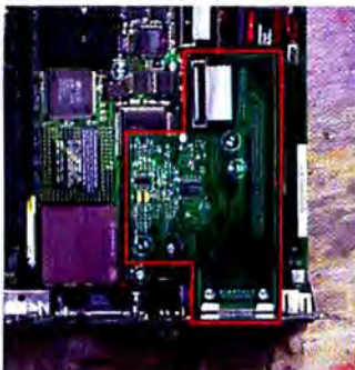
Two daughterboards (outlined) and on-board VGA video let this version of the Quadra 630 run PC programs.
