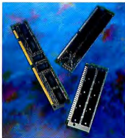
The next generation of Power Macs will use DIMM strips similar to those shown above.
