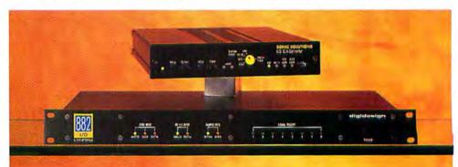
Audio Interfaces High-end audio hardware—such as Sonic Solutions' Sonic A/D-D/A Converter (top) and Digidesign's 882 I/O Audio Interface—include interface boxes that connect to external analog and digital audio gear, as well as NuBus-based DSP cards.
