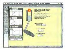
Pumping Iron This simulation of a single-piston engine keeps track of the forces and torques on each mechanical component. But the great strength of Working Model is the scripting facility, which lets designers experiment with different configurations automatically.
