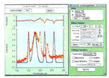
Peak Performance Igor Pro's slick, interactive method for analyzing peaks in experimental data allows you to curve-fit standard mathematical peak shapes to experimental peaks singly or in groups.
