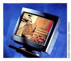
10-bit digital-to-analog converter (DAC) chip and is capable of calculating a total of 10 bits of data for each of the 3 color channels, for a total of 30 bits. Though the LeMans board introduced 30-bit capability more than a year ago (see *Reviews*, October 1994), the PressView 21 SR is the first monitor to take advantage of them. With 30-bit color, you always have the ability to view any of 16 million colors on screen, regardless of your calibration settings.
