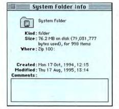
Not Identical Twins How can the same System Folder be 10MB smaller on a Zip disk than on an internal hard drive? The larger the drive, the bigger the allocation blocks it uses to store files—which can add up to a lot of wasted space.
