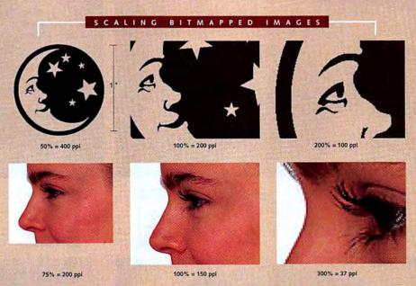
When you scale an image in a page-layout program, the number of pixels in the image doesn't change, so each pixel must get larger or smaller. If the pixels get too large, you get pixelization—the image looks jagged and spotty. When pixels are too small, you waste disk space, RAM, and print time, because you have more pixels than you really need. Past a certain point, the improvement is imperceptible.
