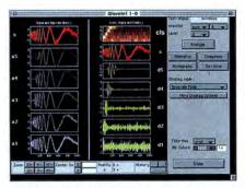
All Quiet on the Wavelet Front The decomposition here shows the MATLAB Wavelet Toolbox isolating and discarding noise from a chirp-type signal.
