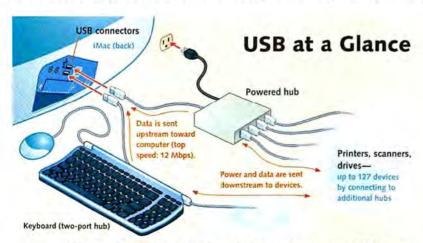
Unlike current Mac serial ports, which are limited to one device per port, USB lets you attach up to 127 different devices at once. To add devices, just add hubs, small devices that give you more places to plug in USB peripherals. The iMac's keyboard itself is a hub, with two ports-one for the iMac mouse, the other ready for some other USB device.
