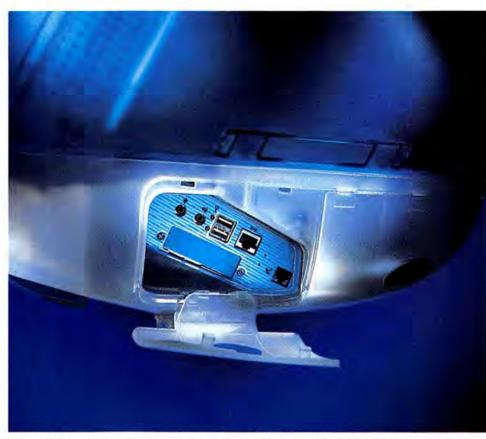
Window to a New World Inside the iMac's side port door are a suite of connectors that prove just how this Mac is not like any other. In addition to audio-in and -out ports (far left) and a phone jack (far right), there's an Ethernet port (second from right). The new faces in this scene are the pair of USB ports (middle), the only means of connecting external peripherals to the iMac. What's most conspicuous is what's not here—no ADB, no Modem and Printer ports, and no SCSI port.
