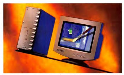
The Cache Advantage Most of the shipping Macs we tested, such as the Umax SuperMac S900/250 shown here, have only a 512K Level 2 cache. The two fastest Macs-Apple's Power Mac 9600/300 and Power Computing's PowerTower Pro 250-each have a 1MB L2 cache, a decided speed advantage.
