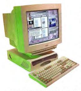
EASY OFF: The Dell OptiPlex GX100 has buttons on its sides that let you remove the case for upgrades.
