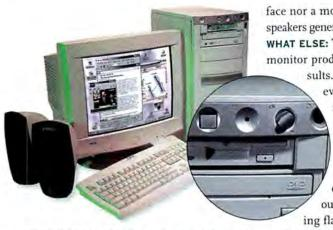
TAKE IT FROM THE TOP: The silver bar at the top of the NEC's PowerMate ES 5250 contains buttons for on/off, sleep mode, and volume control, as well as a headphone jack and an external USB port.
