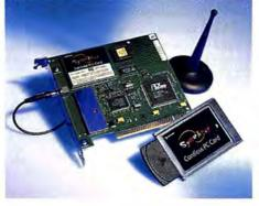
3 Install the wireless add-in card. Turn off your PC and unplug it from the wall. I recommend you wear an anti-static wrist strap (available from electronics stores such as Radio Shack) to prevent static damage to your PC. Locate a free PCI or ISA slot (depending upon
