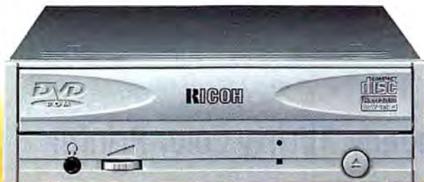
DYNAMIC DUO: Ricoh's MediaMaster MP9060A is both a DVD-ROM and a CD-Rewritable drive, but it costs more than two separate units.
