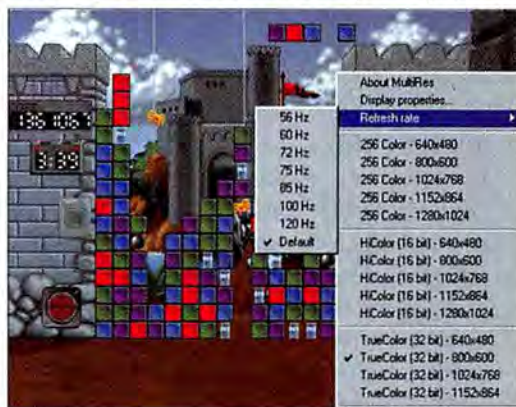
FIGURE 2: MULTIRES allows you to change screen resolution and color depth without system reboots.
