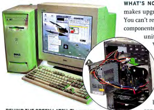
BEHIND THE GREEN LATCH: The power supply on the Dell Dimension L600r swings out for easy access when you press the release mechanism on the case interior (see inset).
