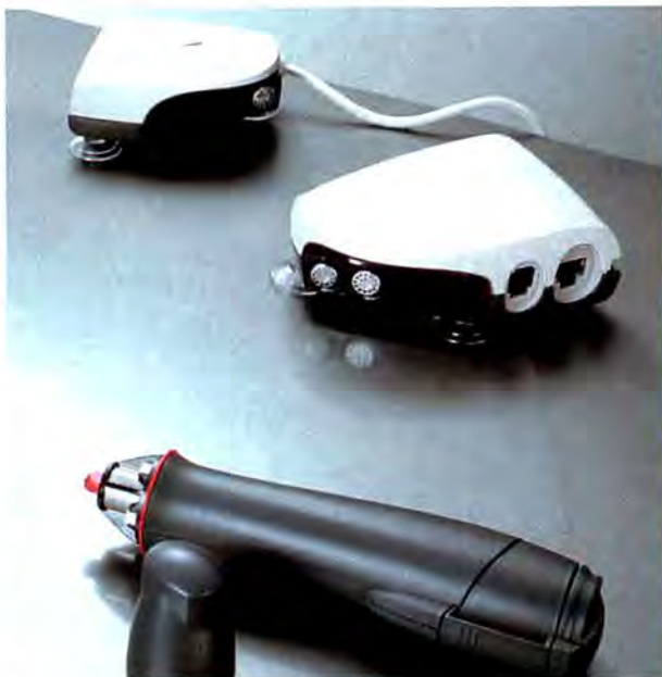
CARRY-ON LUGGAGE: EBeam's hardware—two small pods and sheaths for markers—captures scribbles on conventional whiteboards.
