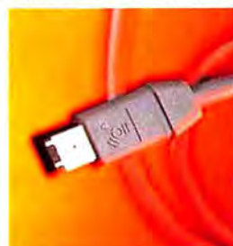
TOP: An IEEE 1394 cable. RIGHT: Adaptec's HotConnect Ultra B945 provides 1394 and SCSI.
