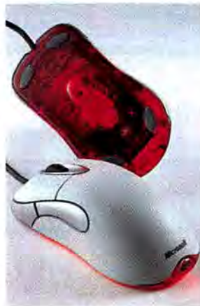
SMOOTHIE: The IntelliMouse Optical has no moving parts.
