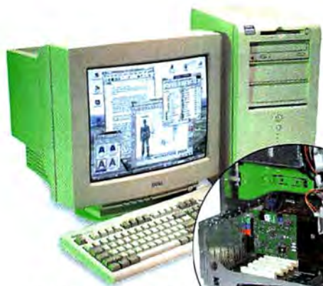
RISE UP: Pull a green lever inside the Dell OptiPlex GX110 and a riser card, which carries the expansion cards, comes out for easy access.
