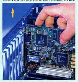
In with the new. Remove your new graphics card from its packaging and carefully insert it into your PC. Press it firmly into the proper slot, and use the screw that you removed in step 3 to secure it. Reconnect the monitor cable, but leave the case off for now.
