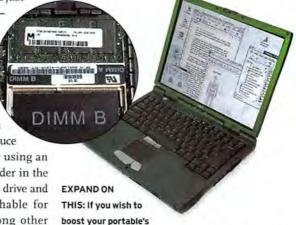
memory, RAM slots on the bottom of the Dell Inspiron 3800 can easily be reached for upgrading.
