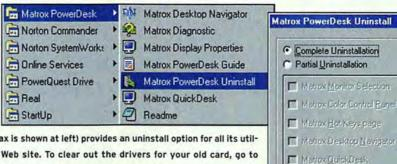
For example, Matrox (whose Millennium G400 Max is shown at left) provides an uninstall option for all its util-Itles and complete uninstall directions on its Web site. To clear out the drivers for your old card, go to Start Settings Control Panel, double-click the Add/Remove Programs icon, and remove any software that's specific to your old graphics card. (If you're not sure about an item, don't remove it!)
