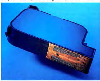
the ribbon and mechanical let- FIGURE 1: INK JET PRINTERS may use over 160 tiny nozzles to create ter heads with a printhead that crisp, near-laser-quality images-but they may require manual cleaning.
