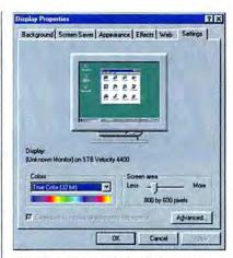
FIGURE 3: AN UNRECOGNIZED monitor's refresh rate is limited to a flickering 60 Hz.
