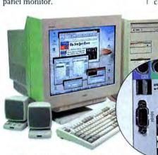
A SINGLE SERIAL: The Dell Dimension XPS B866r provides one serial port and two USB ports for hooking up peripheral devices such as a mouse, an external modem, and a digital camera.
