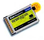
The new 3Com<sup>®</sup> autosensing XJACK<sup>®</sup> connector. For simple 2-in-1 connections through LAN or modem.
