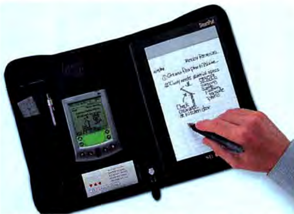
THE SEIKO SMARTPAD allows you to beam the notes and drawings you created on a regular pad of paper into a Palm device.
