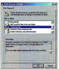
FIGURE 1: THE DISK CLEANUP settings in Windows Me and 2000 automate file deletions.
