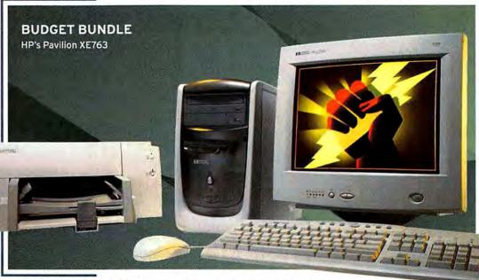
WHAT'S NOT: Game play on Quake III was choppy in high-color mode. The 17inch Optiquest Q71 monitor displayed images and text clearly at a resolution of 800 by 600, but it blurred small text at higher resolutions. When set at 1280 by 1024, the screen suffered from uncorrectable flicker. The system we tested came with limited documentation and no illustrated setup guide.
