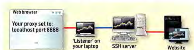
POINTING YOUR WEB browser to "localhost" sends traffic to a port (called a listener) that is configured to open a tunnel from your laptop to the SSH server, where the data will then be forwarded to the destination Website.
