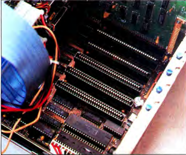
The Portable PC's system board includes one long and four short expansion slots.
