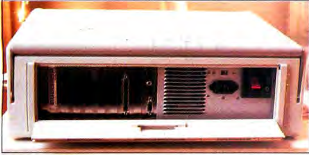
The lowered door opens to reveal the Portable PC's back plane.
