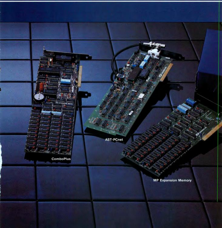
With an AST Research Multifunction Board, you can realize the full potential of your IBM PC or PC-XT without wasting valuable slot space. By combining your memory and input/output requirements on a single card, you can take advantage of more of the capabilities IBM designed into the PC, while leaving space for future enhancements as they are introduced.
