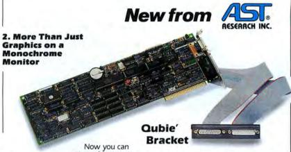
get graphics on an IBM PC monochrome monitor along with parallel port, serial port, and battery powered clock/calendar. It is the ideal solution for those who wish to do graphics using Lotus 1-2-3.™The 720X348 Hercules compatible resolution of the MonoGraphPlus eliminates the eyestrain caused by the IBM graphics adapter with its lower 640×200 resolution.
