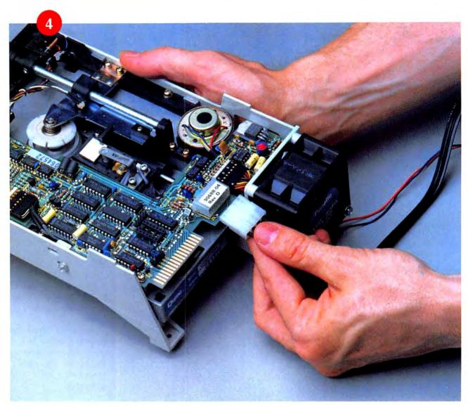
Figure 4. Plug the black disk drive power cable into the four-prong connector on the disk drive. The connector is next to the disk drive's fan.
