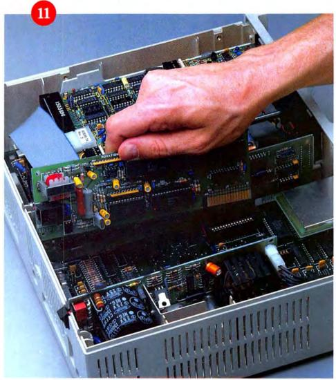
Figure 12. The remaining slot is the longest of the three slots and is for the memory and display expansion board. This board is encased in a metal covering. Once again, be careful not to crimp the disk drive cable and wires when you plug in the board.
