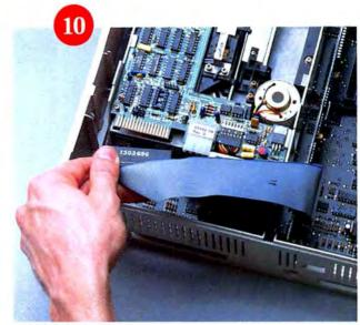
Figure 9. The PCjr has three expansion slots on its motherboard. The slot next to the disk drive is dedicated to the disk drive controller board. Plug the controller board into this slot, but be sure that the board is not crimping the disk drive power cable or fan cord. The controller board. like the two other IBM expansion boards, has notches that provide safe passage for these wires.
