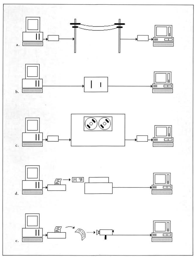
Figure 1: Five methods for converting data to the PC: (a) telecommunications, (b) mainframe conversion software, (c) disk conversion devices, (d) optical char-
