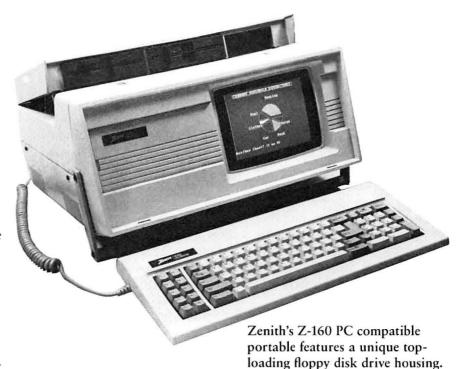
dual half-height 5¼-inch floppy drives, and a system with one half-height floppy drive and a 10.6MB hard disk. The portable comes with either one or two half-height floppy disk drives mounted within a hinged box that occupies the rear three-quarters of the top of the portable. The box flips up when the machine is in use. Both portables weigh 30 pounds and include 9-inch amber monitors. Monitors are not standard equipment for the desktop models. The portables cost \$200 more than the desktops.
