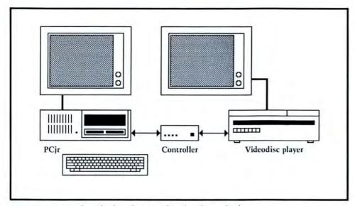
Figure 2: A PCjr and a videodisc player combined with two displays
