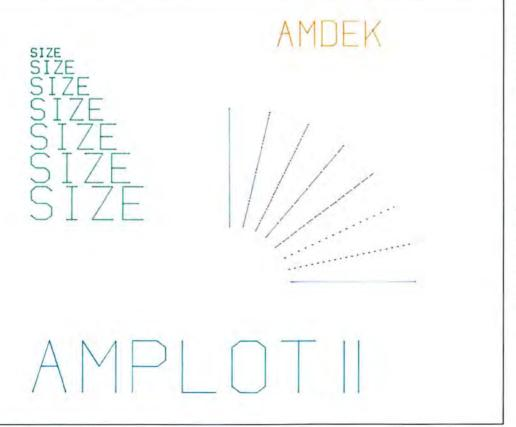
The built-in demonstrations and self-tests for the HP7475 (top right), the DMP29 (top left), and the Amplot II (bottom) plotters. Note that the DMP29 prints out the switch settings for the communications parameters as well as the revision number of the ROM installed in the plotter. -4
