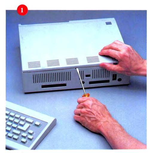
Figure 1. Turn your PCjr off. Disconnect the power supply cord and transformer, the monitor and attachment cable, and any other cables or cords attached to the system unit. Place the system unit on a flat work surface and turn it so the back panel is facing you. Gently pry open the system unit cover with the screwdriver. The PCir has three notches on the back panel for this purpose.
