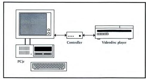
Figure 1: A PCjr and a videodisc player combined with one display
