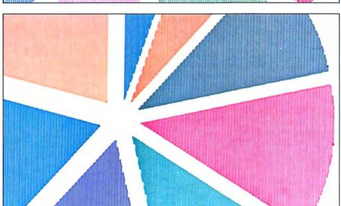
Figure 2: Pie charts drawn by (from top to bottom) the HP7475, the DMP29, and the Amplot II illustrate plotting quality. The HP7475 produces the most even shading and the sharpest lettering.
