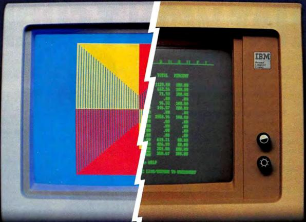
IBM Color Mode plus 640h × 200v - 16 colors 640h × 400v - 16 colors Parallel Port Soft Scroll IBM Monochrome Mode plus High Resolution Graphics 132 Columns Display Parallel Port Soft Scroll
