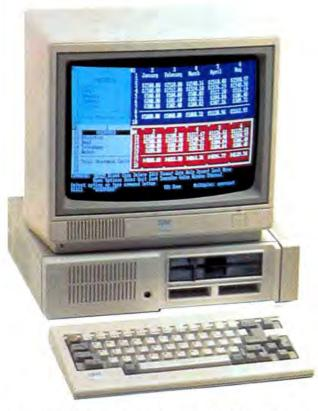
keys are full-size and closely spaced and have character symbols imprinted directly on them. As on the PC keyboard, letter, number, and symbol keys are white, and operation keys are gray. The keyboard also includes some nice extra touches, such as small ridges marking the J and F home position keys so they can be found by touch.
