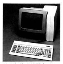
The Televideo PM Workstation, a PC-compatible diskless computer designed for TeleVideo's Personal Mini multiuser system
