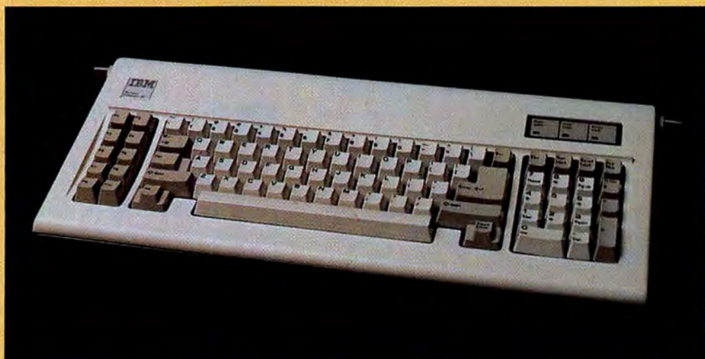
Figure A: The AT sports a redesigned 84-key keyboard, complete with enlarged <Enter> and <Shift> keys and a segregated cursor keypad.
