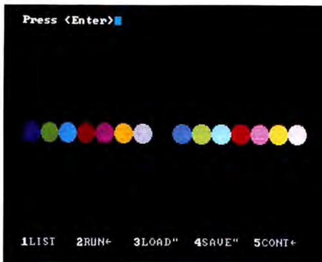
Figure 1: The program in Example 2 draws circles in each of the 16 colors available in SCREEN 5. With the PALETTE statement you can instantly change the color of any circle or even make a circle appear to move across the screen.
