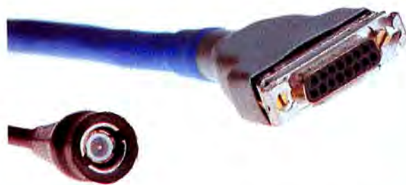
Ungermann-Bass's Net/One relies on a thin Ethernet coaxial cable (bottom); the transceiver cable at the top links the 3Com EtherSeries network with a transceiver.
