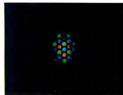
Figure 2: A pixel, composed of several phosphor dots, is the smallest screen area that the PC's graphics controllers can normally address.
