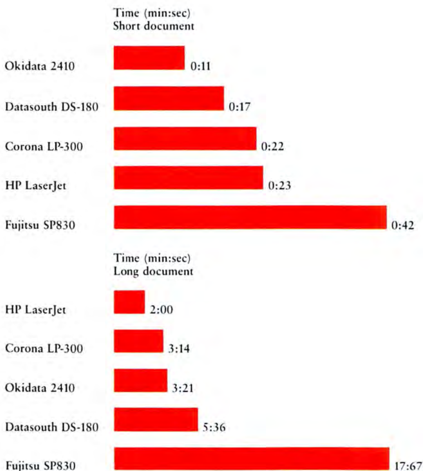
Figure 1: Speed comparison for the Corona LP-300 laser printer; the Hewlett-Packard LaserJet laser printer; a high-speed dot matrix printer (Okidata 2410, $2475); a medium-speed dot matrix printer (Datasouth DS-180, $1395); and a daisy wheel printer (Fujitsu SP830, $2295). The long document is 600 lines; the short document is 25 lines.
