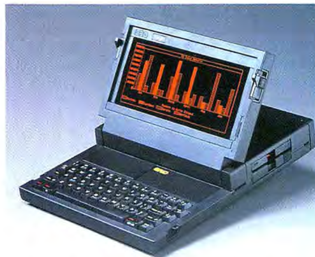
Figure 2: GRiD system's GRiDCase 3 flaunts a “sexy” plasma display. New technologies are bringing plasma displays within reach of their most elusive goals: lighter weight and lower power consumption.
