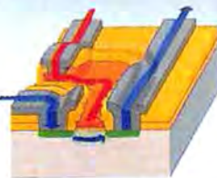
How a transistor operates as a switch.
