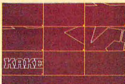
Screen C: Establishing key frames, the first step in the animation process. Real-time previews of the action can only be done with a wire-frame model.
