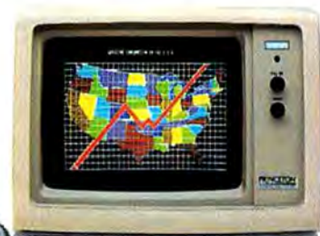
SR-12P. PGS's top of the line RGB monitor 640x480 lines noninterlaced - .26 mm dot pitch - Analog input allows for the display of 4,096 possible colors -Compatible with IBM Professional Graphics Adapter -Nonglare screen -$999
