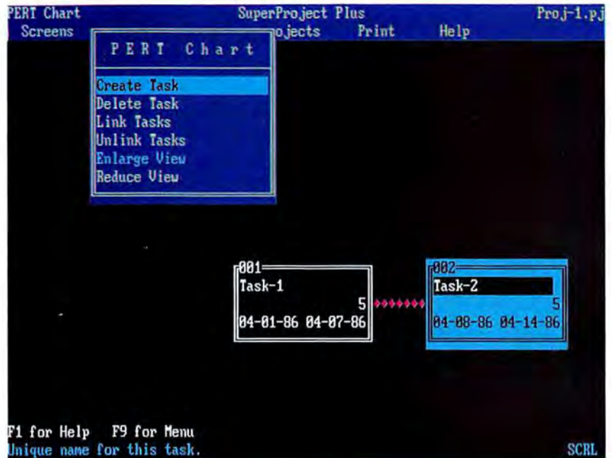
Screen 2: The PERT Chart menu with pull-down options and a sample of two tasks linked by the critical path
