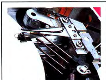
Super Tough — The Gold-Card's automatic head unloading mechanism is key to its high reliability and makes it perfect for portables.
