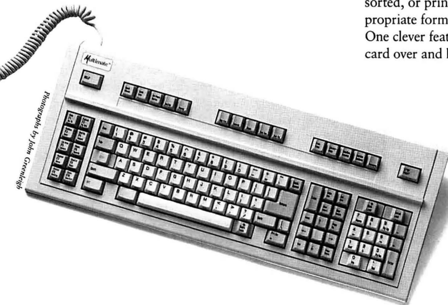
Figure 2: Multimate's optional keyboard works with both Advantage and MultiMate 3.3 . The keyboard provides 10 PC-compatible keys on the left, 17 Wang-like keys on the top, and 14 additional function keys. Twenty-two of the keys are programmable.
