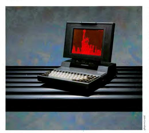
Offering an eyepopping gas plasma display, Toshiba's 14pound T3100 gives you the freedom to take 80286 power almost anywhere. And with 640K RAM, a 10MB hard disk, and an 8-MHz switchable clock, you won't have to swap performance for mobility.
