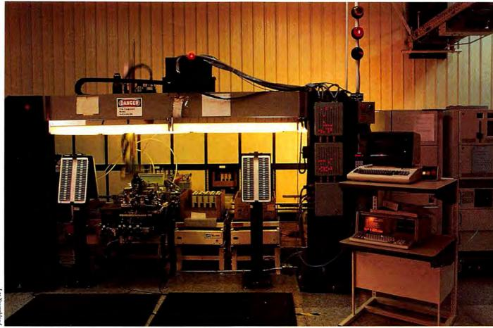
Machine vision dictates specific lighting conditions, as this robotic assembly module indicates. The Portable PC at right collects parts inventory data and passes build instructions between robot controllers and the control room.
