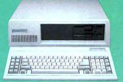
Includes 8088-2 Dual Speed (4.7 MHZ-7.4 MHZ) unit, 640 K RAM, 360 K Floppy Drive W/Controller, AT\* Style Keyboard, 135W Power Supply, MS-DOS 3.1 W/Manual, System Manuals, Full 18 Months Warranty, Run all major software for IBM-PC\* and PC/XT\*.
