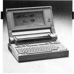
Beneath its sleek exterior, Wang's compact portable packs a hard disk drive and a thermal transfer printer.
