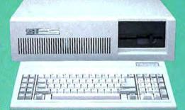
Includes 80286-Based 8MHZ unit, AMI BIOS, 512K on 1MB Monther Board, 1.2 MB Floppy Drive, W.D. Hard/Floppy Controller, Clock/Calendar W/Battery Back Up, AT Style Keyboard, 200-W Power Supply, MS DOS3.1 W/Manual, System Manuals, Full 18 Months Warranty, Run all major software for IBM-PC/AT\*
