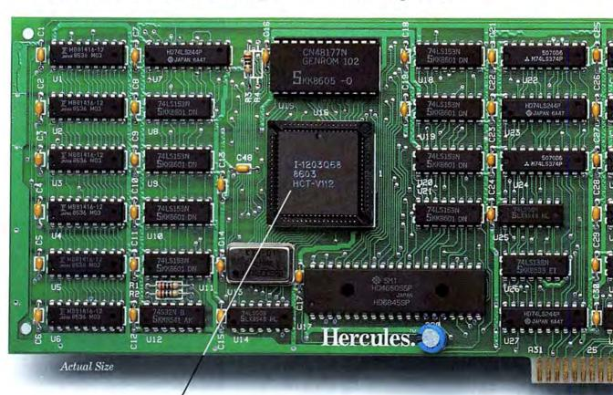
The heart of the Graphics Card Plus: the V112 microchip, Hercules' next generation video processor that makes the RamFont mode possible.
