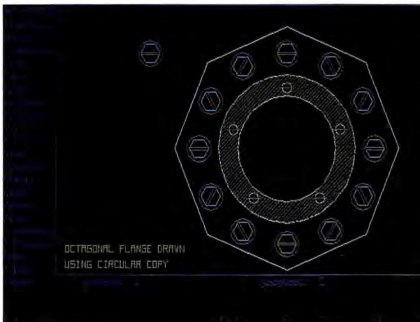
Screen 3: This drawing of a flange illustrates VersaCAD 's circular-array copy function. The top view of a bolt head and washer shown in the upper left was automatically reproduced in 30-degree increments around the flange with a few keystrokes, as were the five holes on the central ring. Note that the bolt heads were rotated 60 degrees for each successive location, while the holes were not rotated.
