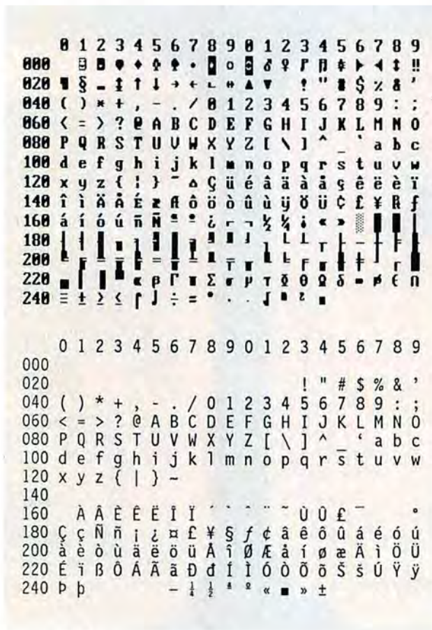
Figure 1: A comparison of the character sets used by the IBM Monochrome Display Adapter (top) and the HP LaserJet (bottom). Although both use the same keyboard characters, graphics characters (ASCII 127 to 256) are decidedly different.
